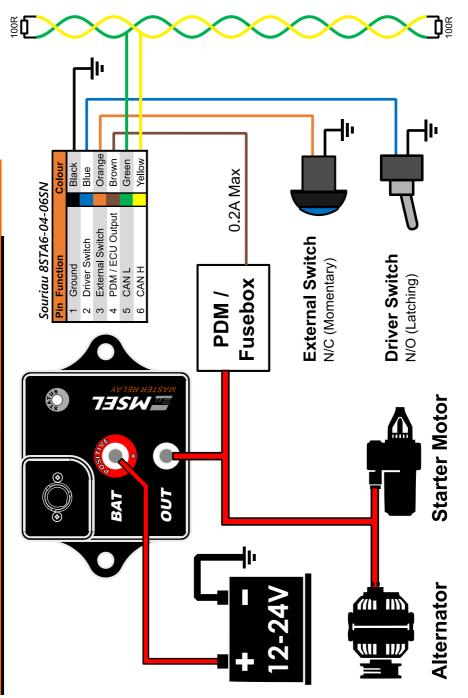
Figure 1: Connection Diagram
